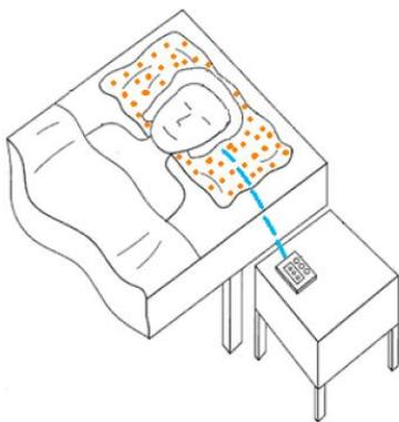
ChronoWake is designed to monitor the user's EEG signals throughout the night via imperceptible sensors embedded in the pillow. The gathered signals are then wirelessly transmitted to the processing unit, which perform analysis and determine what sleep stage the user is in, and consequently, the ideal time to wake up.
